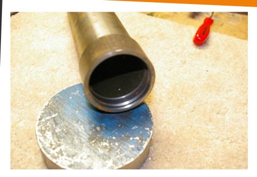
The ramp to the tube needs to also be chamfered, as this location is where the o-rings slide in (piston and the bronze cap ring) We can't risk cutting those after all this work has been done.
