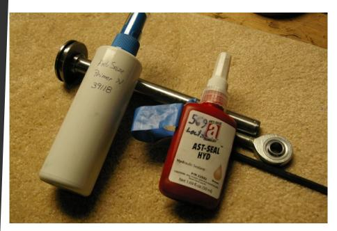
The two numbers for sealant to use. Loctite is 569 with primer 39118 or commonly called Primer N or the spin off of loctite is this product AST-SEAL HYD
