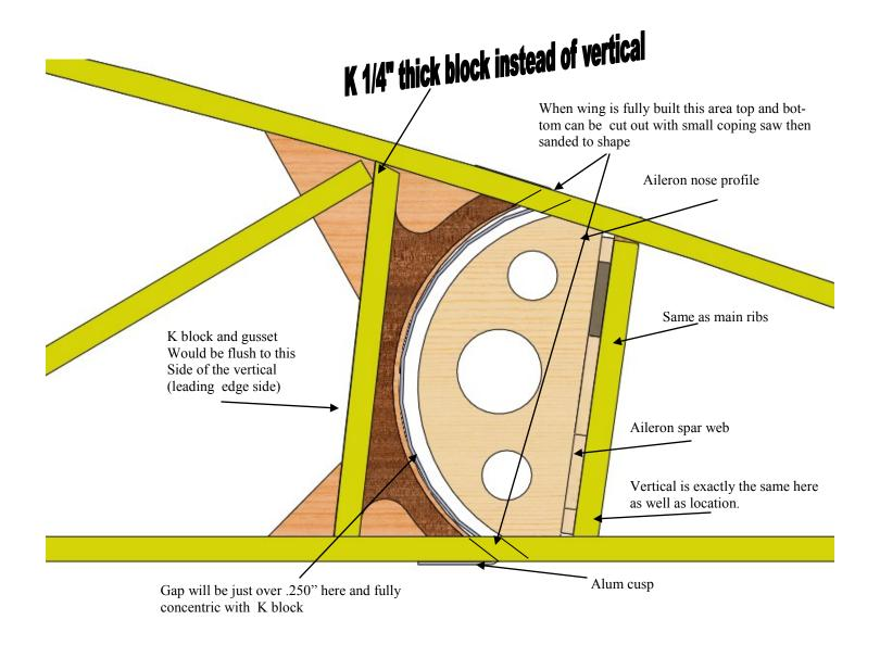
All shapes and dimensions based on easy part cut outs following supplemental plans only. Aileron is the same size as the original plans only the build procedure is slightly different.
